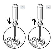
[1] Press in the stem of the MO with a pointed object or screwdriver.The pilot valve switches and actuates the main valve.
