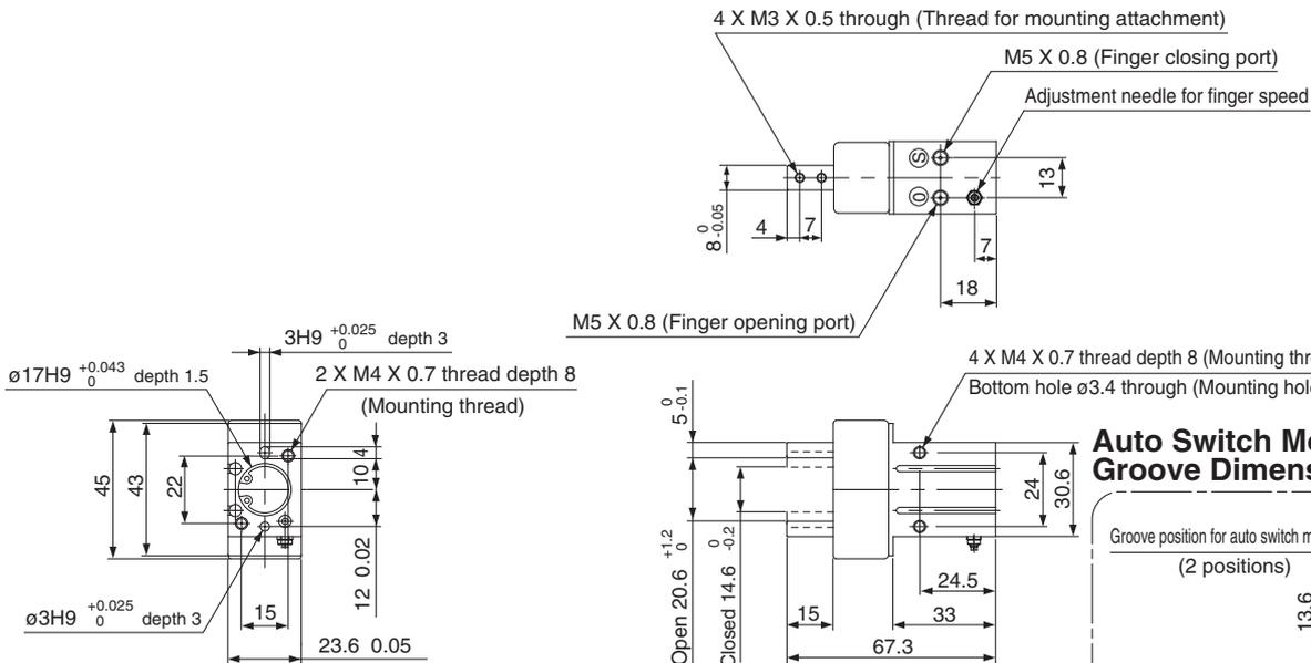
Note) For single acting, one port is used as a breathing hole. Adjustment needle for finger speed is used as a plug.
