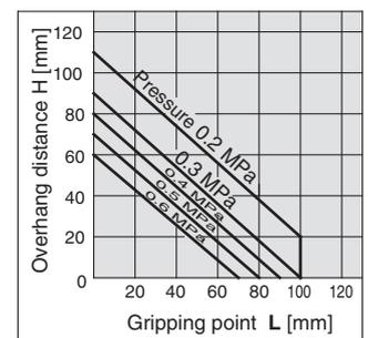
Note) Distance to the gripping point L of single acting type is shortened by spring return.
