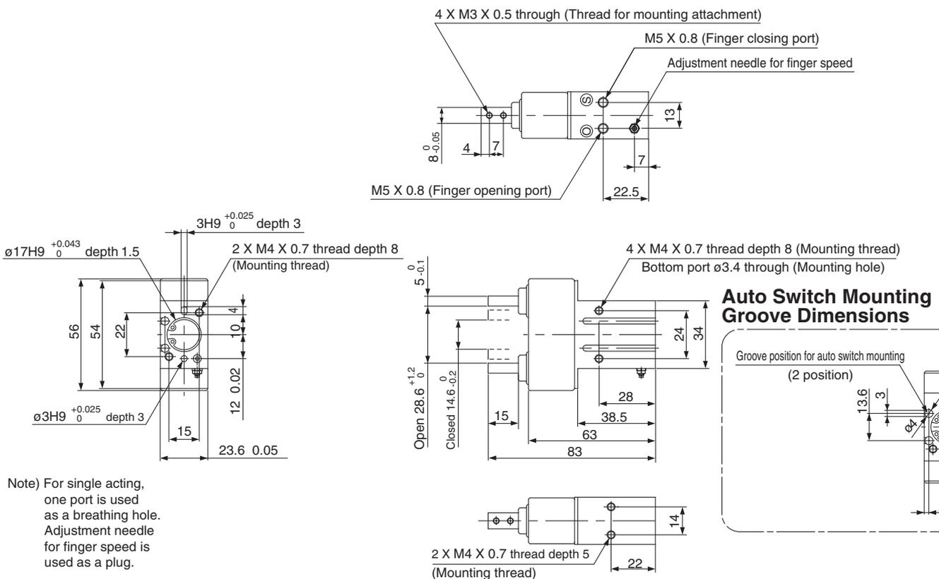
Note) For single acting, one port is used as a breathing hole. Adjustment needle for finger speed is used as a plug.
